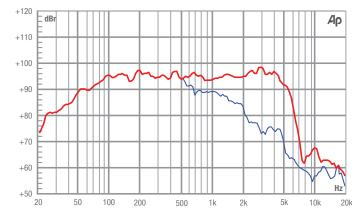
A.E.S. power handling test. Pink noise bandpass filtered at 12 dB per octave with cutoff frequencies of 50 Hz and
